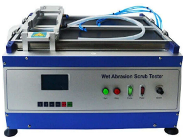
Figure 8. Sheen Scrub Tester used in the scrub resistance test for current acrylic paint formulation.
